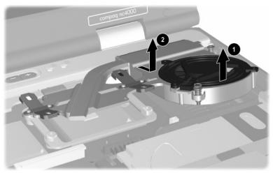
Removing the Heat Sink
